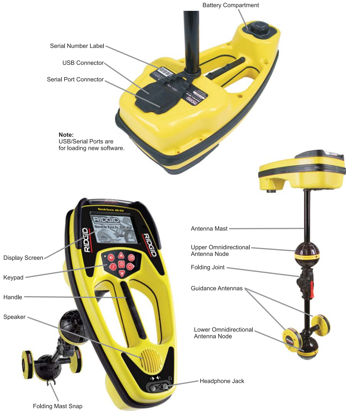
Figure 1: SR-60 Components
